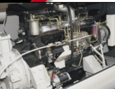
248 hp Isuzu A-6SD1T-QB-01 engine
